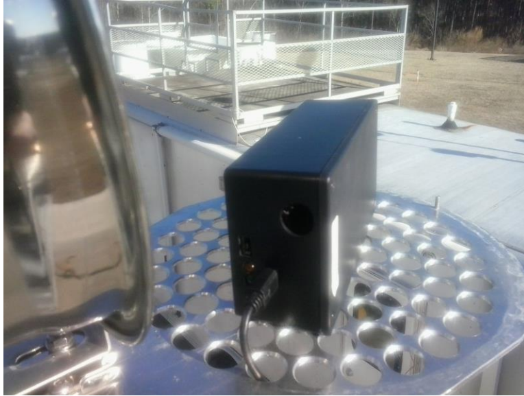
Figure 2.1.8-1. Sensaris Eco PM oriented in its shelter with the lid up.
