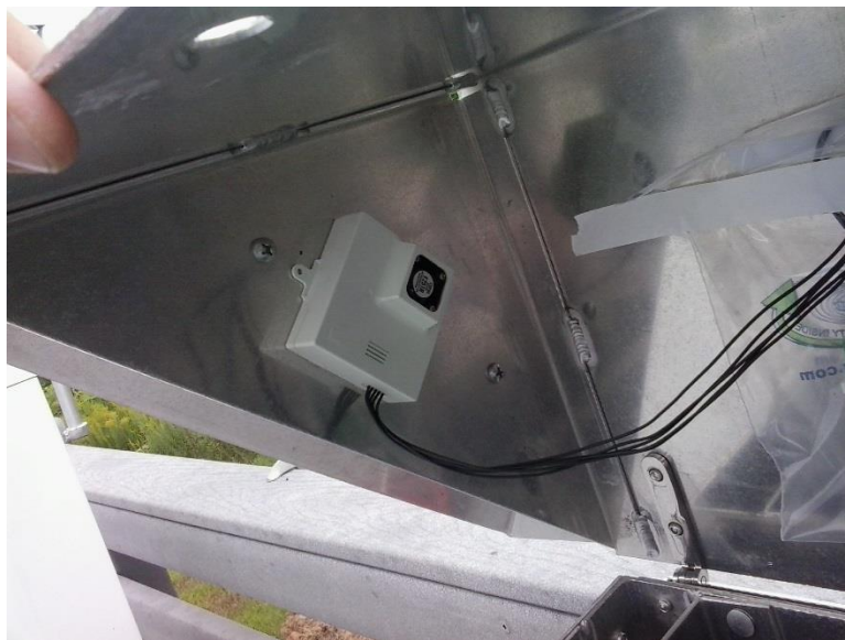
Figure 2.1.9-1: Shinyei in a Hi-Vol shelter. Note that the lid to the Hi-Vol shelter was closed during sampling.
