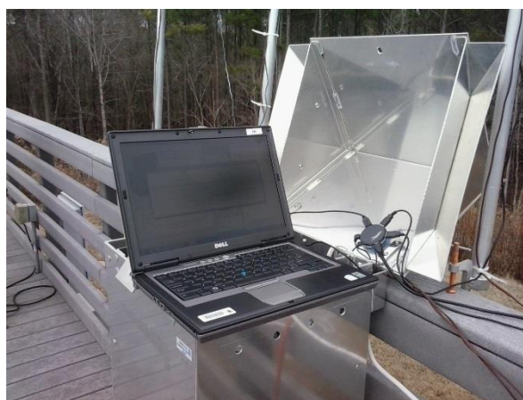
Figure 2.1-2. Hi-vol shelter opened with laptop displayed (left) and with wiring and laptop inside (right).
