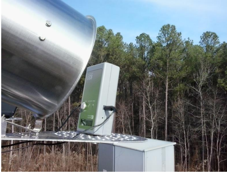
Figure 2.1.6-1. Met One model 831 oriented in its shelter with the lid up.
