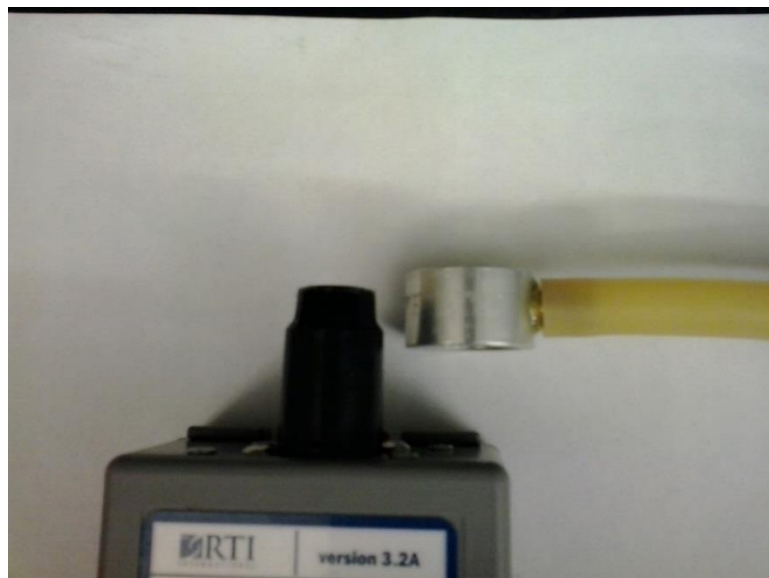
Figure 3.6.1-10. RTI MicroPEM inlet alongside the gasketed cup which serves as an attachment point for the zero air filter.
