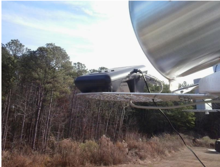
Figure 2.1.5-1. Dylos DC1100 oriented in its shelter with the lid up.
