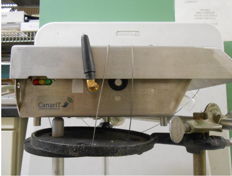
Figure 2.1.2-1. AirBase CanarIT attached to laboratory stand via bailing wire.
