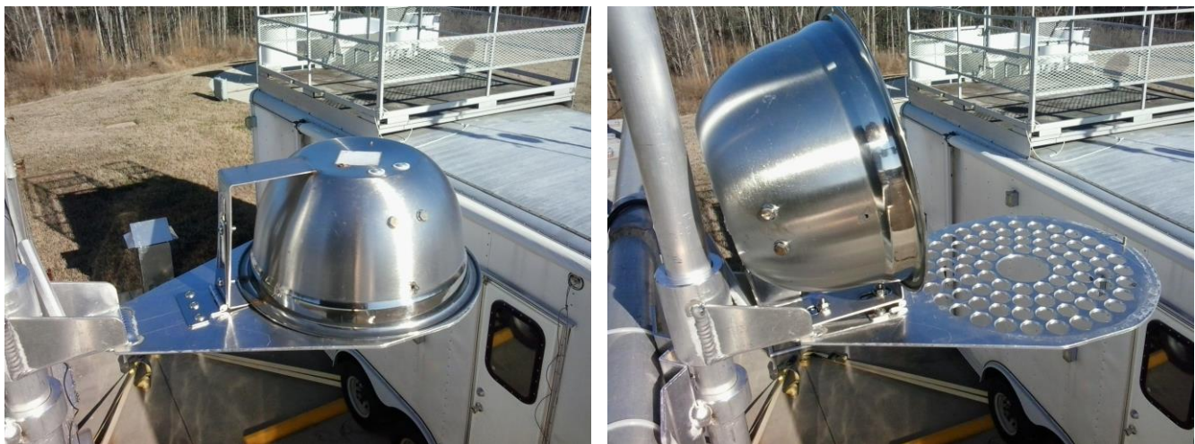
Figure 2-1. “Bowl on pole” sensor enclosure in closed (left) and open (right) positions.
