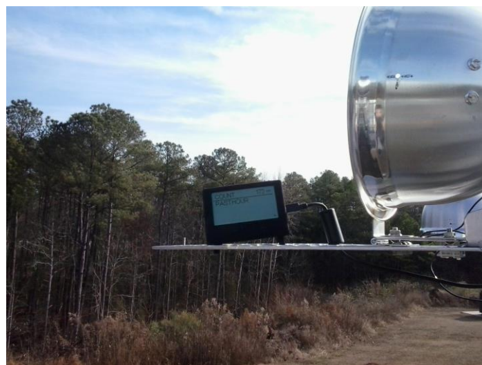
Figure 2.1.4-1. Carnegie Mellon Speck oriented in its shelter with the lid up.
