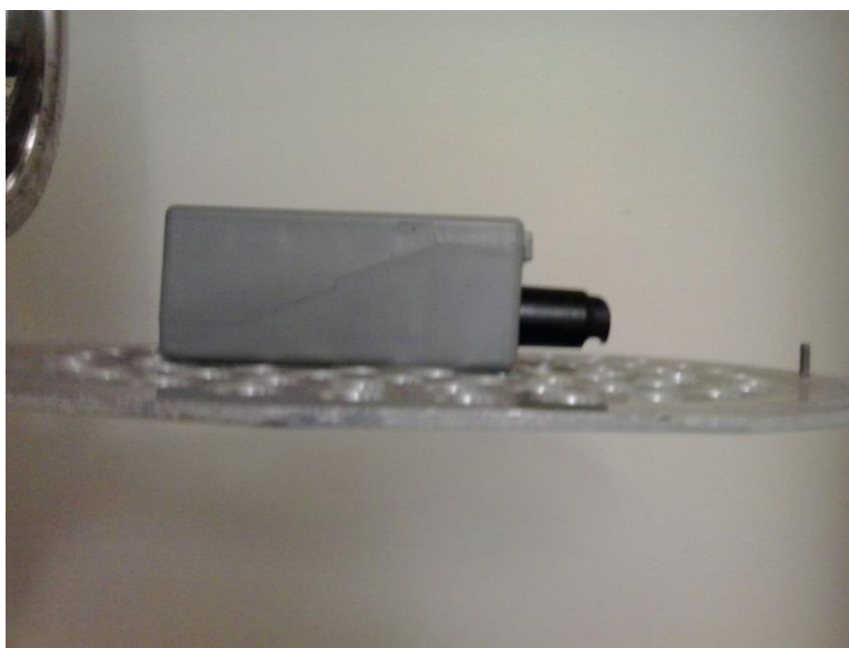
Figure 2.1.7-1. RTI MicroPEM orientation on the plate of a bowl-on-pole shelter.
