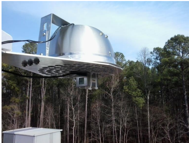
Figure 2.1.3-1. CairClip PM sensor suspended beneath shelter grating.
