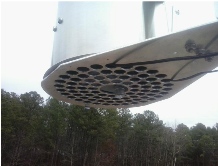
Figure 2.1.6-2. Met One model 831 oriented in its shelter with the lid down.
