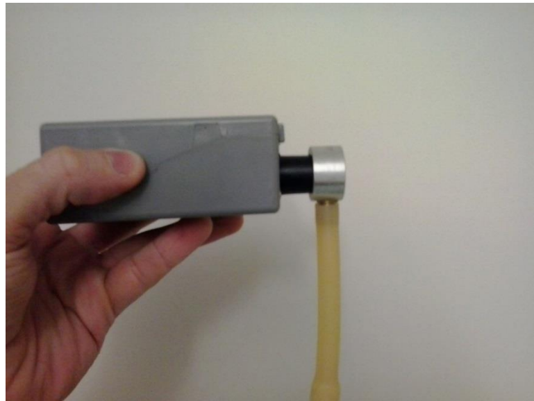
Figure 3.6.1-9. RTI MicroPEM with zero air filter attached.
