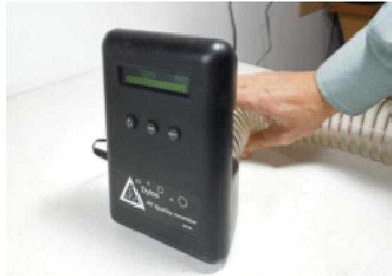
The DC1100 Pro Air Quality Monitor with PC Interface is \$289.99. It can detect particles down to 0.5 microns in size. The large particle size is calibrated to 2.5 microns and above. The LCD screen shows small and large particle counts with a bar graph that shows the actual count readings. There are multiple modes that can be used to evaluate the air quality such as minute, hour and day. The data for all of the monitors is stored up to 30 days and can be sent to a PC for graphing and analysis.
